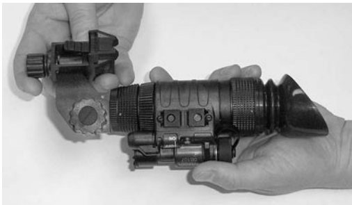
Figure 3-3 Attaching ATN NVM-14 to Headmount Adapter
